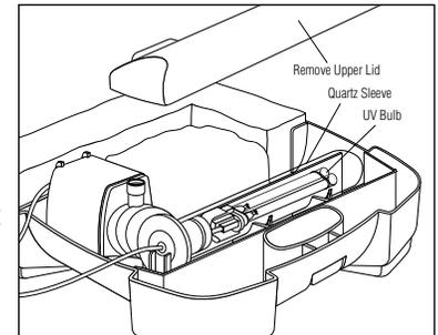
**5. To Change UV Bulb:** For best efficiency UV bulb should be replaced yearly. (Approx 9000 hours of use). Disconnect both pump and UV. Remove the upper lid. Remove the bulb lid. Using a screwdriver, extract the quartz sleeve and UV bulb and replace with a new one available from your dealer. Reassemble all parts making sure that all gaskets in the bulb cap are placed correctly.
